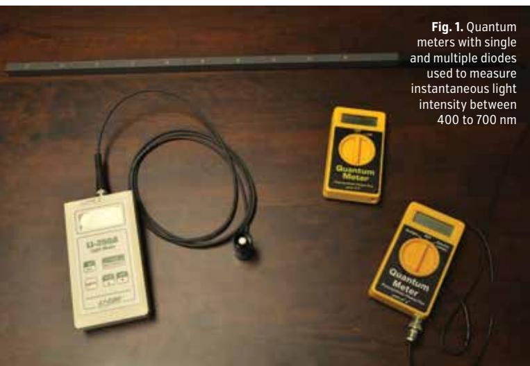
**Fig. 1.** Quantum meters with single and multiple diodes used to measure instantaneous light intensity between 400 to 700 nm
